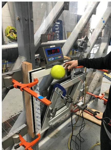
Photo No. 2 Specimen #1 under load with 5" rigid sphere test
